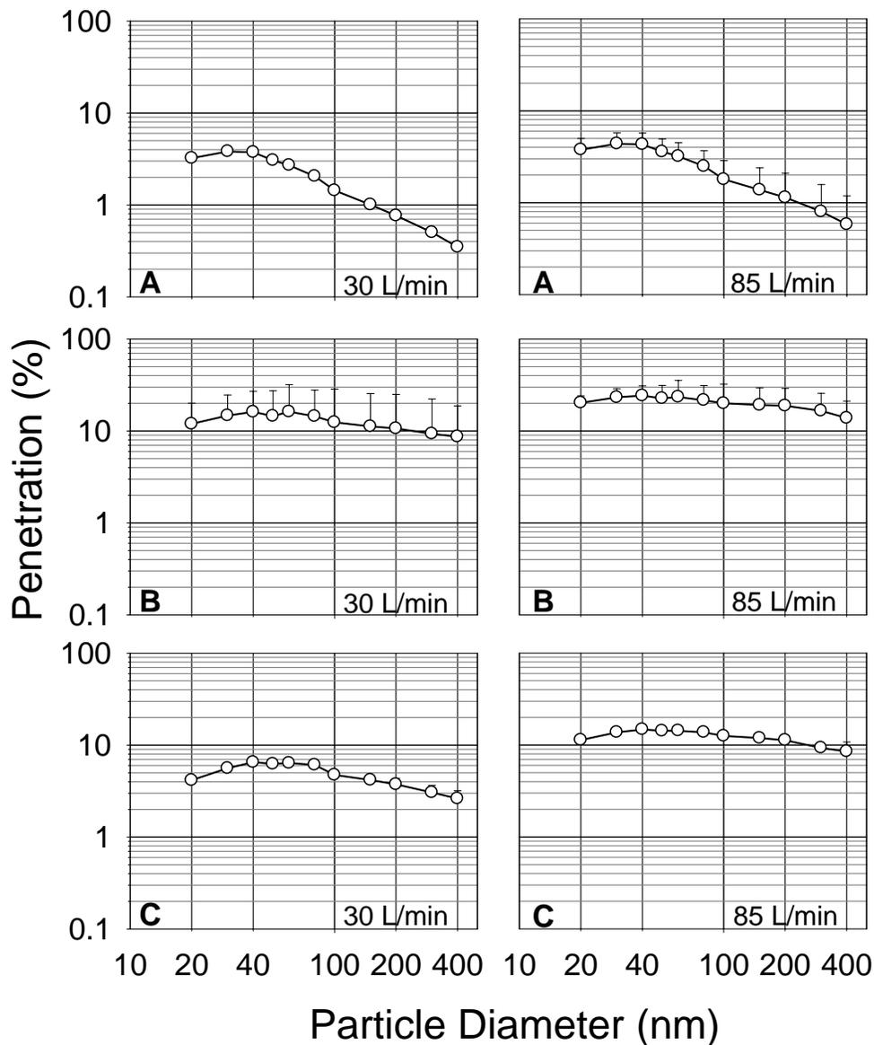
**Figure 2. Penetration levels at 11 different monodisperse particle sizes measured using the monodisperse aerosol test (MAT) method for one low (A)- and two medium (B)-penetration category dust mask models at 30 and 85 L/min flow rate.**
