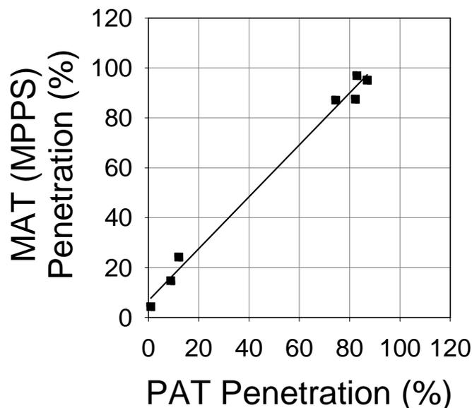
**Figure 4. Correlation of the penetration levels from the polydisperse aerosol test (PAT) method and MPPS aerosol penetrations from the monodisperse aerosol test (MAT) method at 85 L/min flow rate for the seven dust mask models. ( $r = 0.99$ )**
