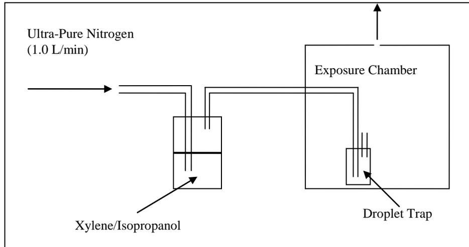
Figure 1. Isopropanol and xylene vapor exposure setup.
