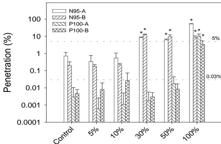
**Figure 2: Polydisperse aerosol penetrations of electret FFRs treated with different concentrations of isopropanol. Bar represents an average of three samples. Upper error bar is at the 95% confidence level ( $n=3$ ). Dashed lines represent NIOSH allowed maximum penetrations for N95 (5%) and P100 (0.03%) FFRs. \* Significantly ( $P < 0.05$ ) different from controls.**
