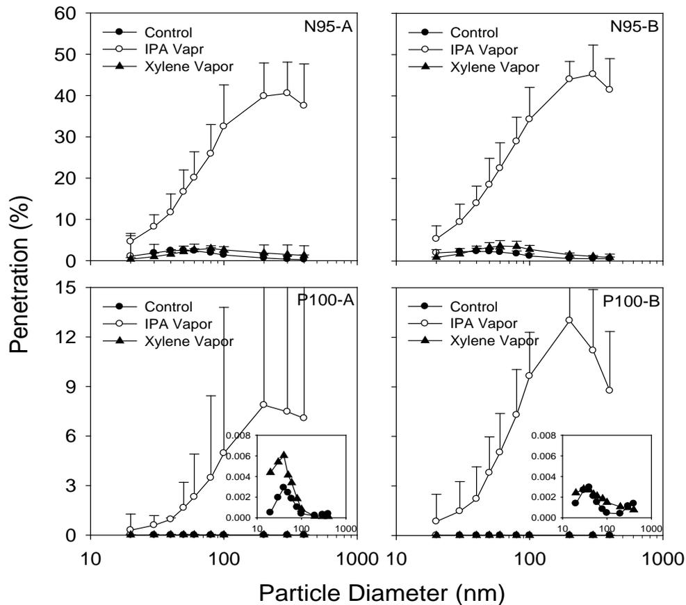
**Figure 6: Penetrations of monodisperse NaCl (20–400 nm) particles through electret N95 (top row) and P100 (bottom row) FFRs from two manufacturers (A and B) at 85 L/min after 8 hour exposure to IPA (open circles) and xylene (solid triangles) vapors. Error bar represents the 95% confidence interval (n = 3). Insets in bottom panels show penetration curves for control and 8 hour xylene exposure for the P100 FFRs.**
