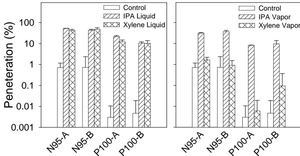
**Figure 4: Polydisperse aerosol penetrations for electret N95 and P100 FFRs at 85 L/min after exposure to IPA and xylene liquids (top) and vapor (bottom). Error bar represents the 95% confidence level (n = 3).**
